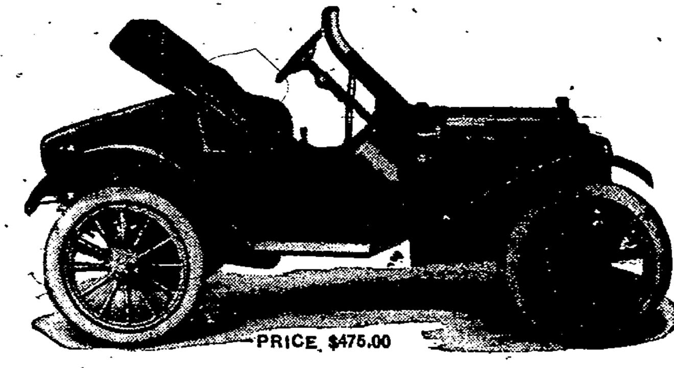
THE MOST POPULAR AND CLASSY FOUR CYLINDER RUNABOUT ON THE TENSION MAGNETO. FULL ELLIPTIC SPRINGS. WHEEL BASE 90 INCHES. 30x3 INCH TIRES. STANDARD EQUIPMENT AND FINISH,
