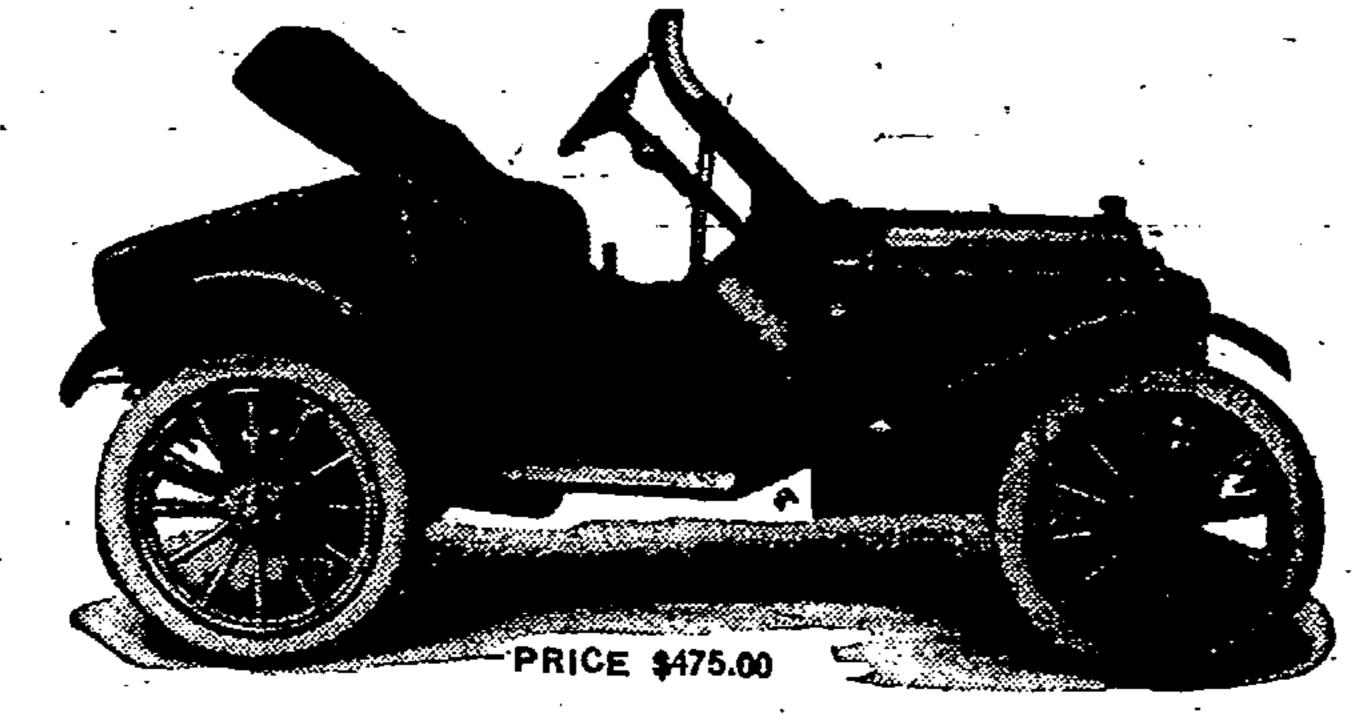
THE MOST POPULAR AND CLASSY FOUR CYLINDER RUNABOUT ON THE MARKET. GEARLESS TRANSMISSION, THERMO-SYPHON COOLED. BOSCH HIGH TENSION MAGNETO. FULL ELLIPTIC SPRINGS WHEEL BASE 90 INCHES. 30x3 INCH TIRES. STANDARD EQUIPMENT AND FINISH.
